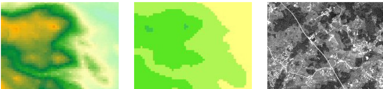
Figure 4. Continuous data (raw elevation values), discrete data (elevation classes), and image data (satellite image) represented in rasters.
