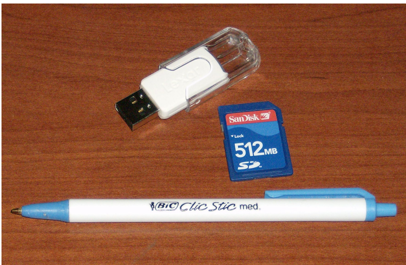
Figure 5. Non-volatile solid-state memory devices. Lexar 2 GB “thumb drive” (left) and SanDisk 512 MB Secure Digital Card (right). Pen is shown for scale.
