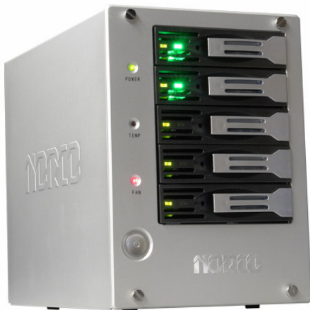
Figure 9. The Norco Technologies DS-500 5-Bay Hot Swappable SATA RAID Storage Array, which contains a hot spare. Notice the levers on each drive face that allow the rapid removal of each drive (Source: http://www.norcotek.com/item_detail.php?categoryid=8&modelno=ds-500 )
