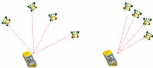
Figure: A good and poor satellite configurations
