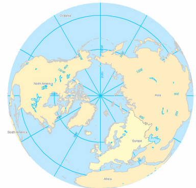
Figure: Orthographic planar - - the projection center at infinity and opposite to a plane surface
