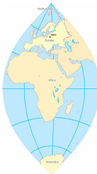
Figure: Conformal Transverse Mercator (cylindrical by shape of graticule and transverse by aspect of developable surface)
