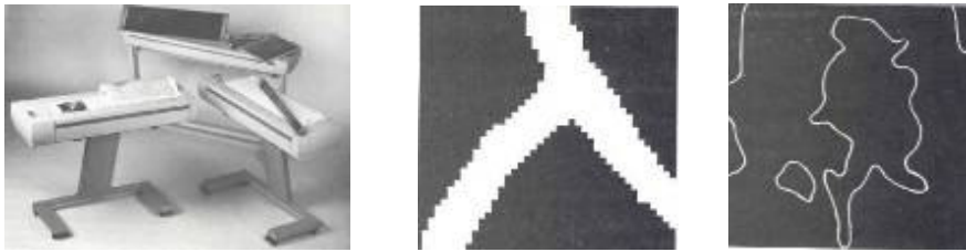
Figure: Equipment for automatic vectorisation, raster lines and derived vector lines
