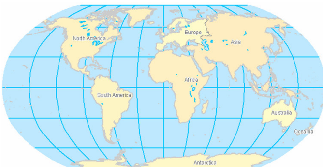
Figure: Pseudo Cylindrical Robinson projection provides solution for the “Greenland via Australia Problem” – relative sizes of the landmasses are preserved
