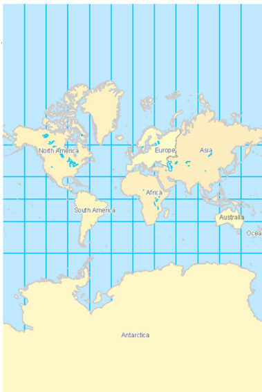
Figure: Conformal Mercator (cylindrical by shape of graticule) projection. Greenland looks larger than Australia
