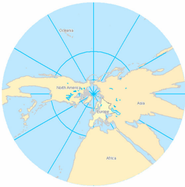
Figure: Gnomonic planar - the projection center is located in the center of globe
